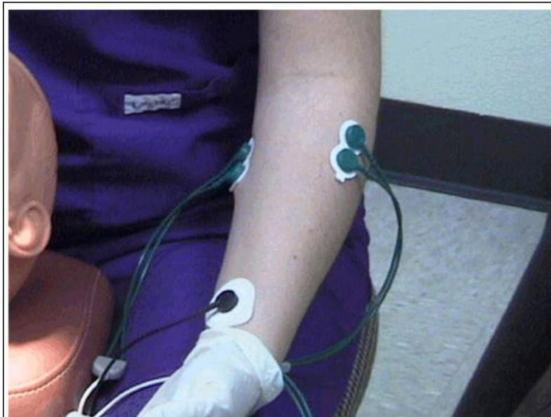
**Figure 2.** Bipolar sensor electrode configuration, used with a single circular electrode placed on the dorsal side of the wrist. The electrode on the upper right is on the *extensor digitorum*, the electrode under the glove is on the *flexor pollicis brevis*, and the electrode on the upper left is on the *flexor digitorum superficialis*. The electrode directly above the glove is the ground.
