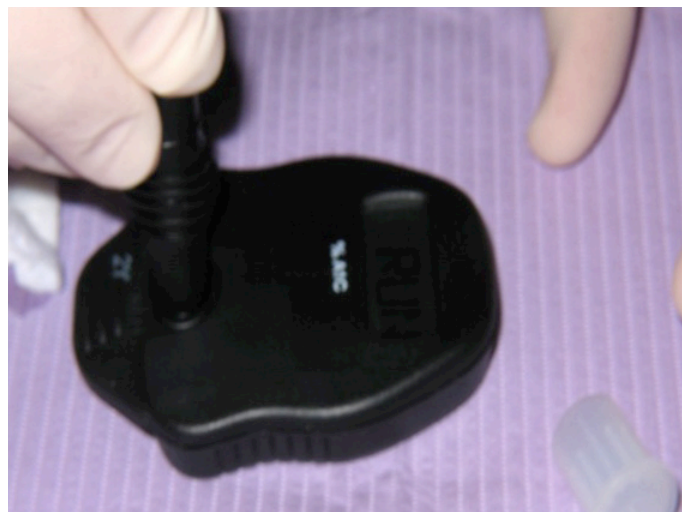
Figure 4C: Transfer of the Blood Solution to the Test Cartridge in the Test Monitor
