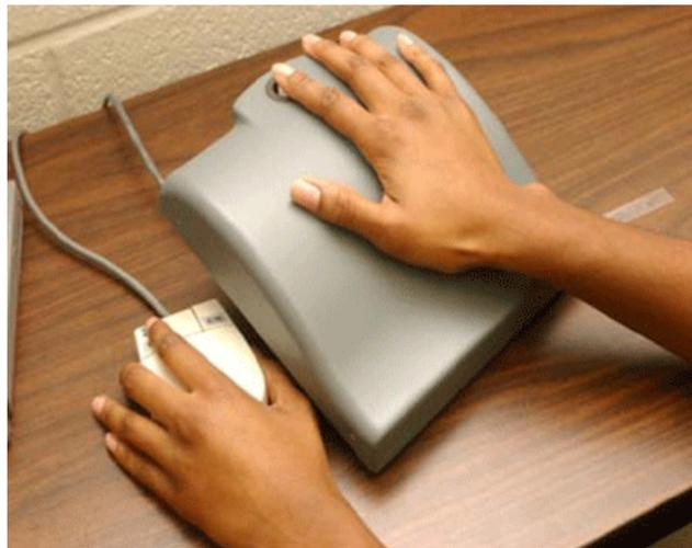
**Figure 3 .** Vibratory Unit with Mouse.
